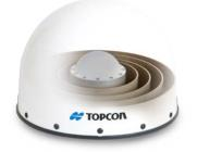
The CR-G5 is a choke ring antenna based on Topcon's TA-5 full spectrum GNSS antenna element. The TA-5 antenna element utilizes an array of vertical convex dipoles. This antenna provides Full Wave tracking technology for existing and future GNSS signals.
