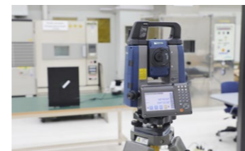
Auto-tracking durability test against rotating object.
